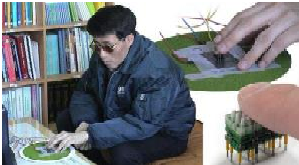
A blind person uses the dielectric elastomer EAP based refreshable Braille display developed at Sungkyunkwan University, South Korea. (Credit: HR Choi, Sungkyunkwan University, South Korea)
