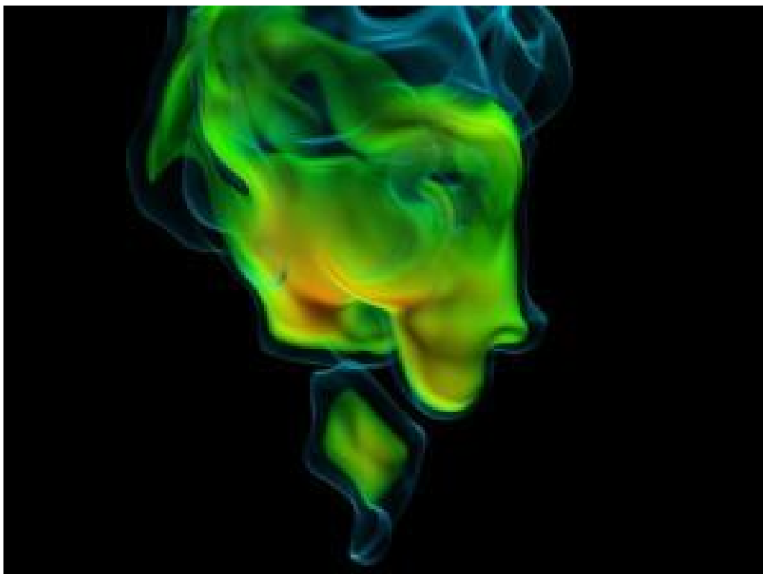
Volume rendering of hydroperoxy (HO 2 ) radical concentration during autoignition. The red colouring indicates a high HO 2 concentration. The little green "bubble" below is about to auto-ignite. (Credit: Photo: LAV/ETH Zurich)
