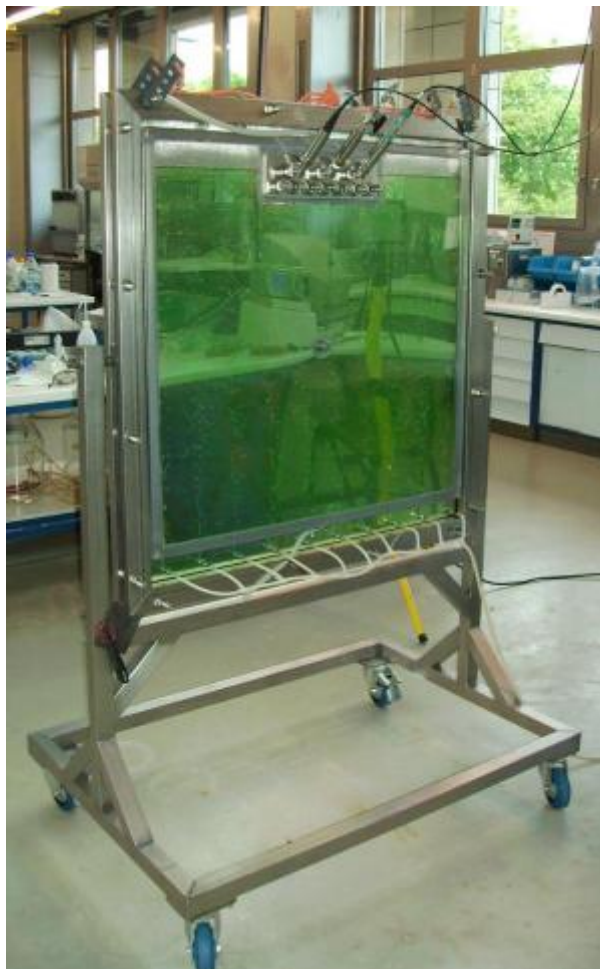
Newly developed plate reactor for an optimum light management in the cultivation of microalgae. (Credit: Photo by Florian Lehr)
